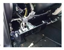
2---Remove 2 10 mm bolts holding lower dash finish panel and carefully pull off
