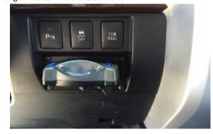
5---Install wiring for P2 mount per instructions with P2, Plug in all switches and reinstall all panels. Done!
