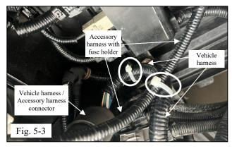
(f) Turn vehicle harness up and apply (1) zip tie to secure with other vehicle harness and (1) zip tie to secure accessory harness with vehicle harness (Fig 5-3).
