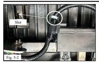
(e) Thread zip tie through the slot shown in (Fig. 5-2) to secure fuse holder.
