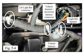
(g) Apply (3) zip ties to secure the light bar harnesses against the accessory harness (Fig. 5-4).
