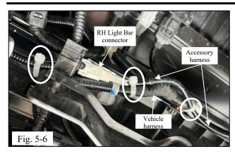
(i) Move to the passenger side. Apply (3) zip ties in location shown in (Fig. 5-6) to continue to secure accessory harness against vehicle harness.
