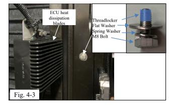
(d) Install M8 bolt, spring washer and flat washer according to the sequence as shown socket with extension (Fig 4-3).
